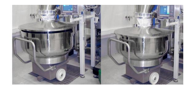
"It doesn't let anything through. The gap between the bowl and the scale is also completely closed, so there is no dust inside."
