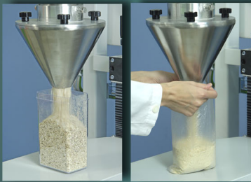
Fillermatic is suitable for all types of powders and granules. The product can be packed in to boxes, pouches etc.
