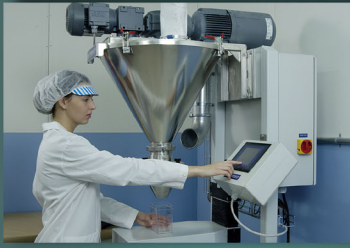
Icon-based touch screen interface makes Fillermatic extremely easy to use.
