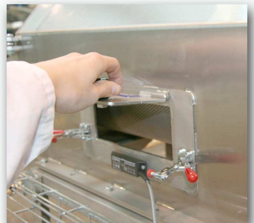
Pic 2. The sifter screen's condition is easily inspected from the hinged inspection hatch.
